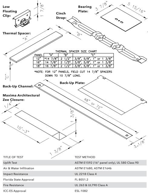
All testing conducted with a Galvolume® substrate.
